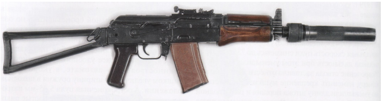
Pic. 20 AKS-74ub with PBS-3 suppressor - a weapon which turned to be a failure due to low effectiveness of the 5.45 mm subsonic ammunition.
