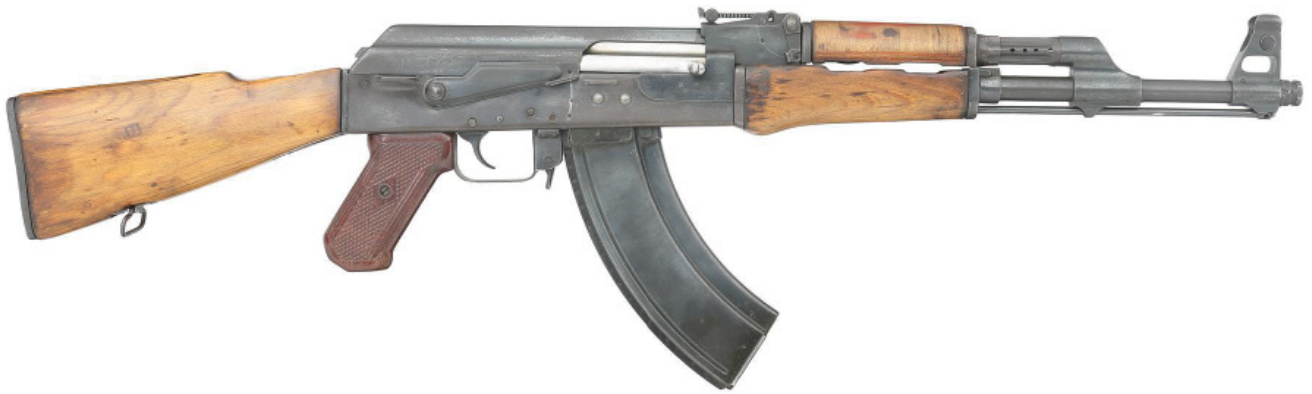
Pic. 10 AK 1951 with early stamped receiver
