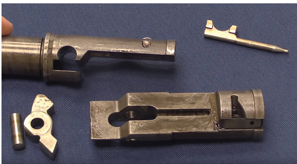
Pic. 16 Kiraly 39M SMG, with two part bolt and lever
