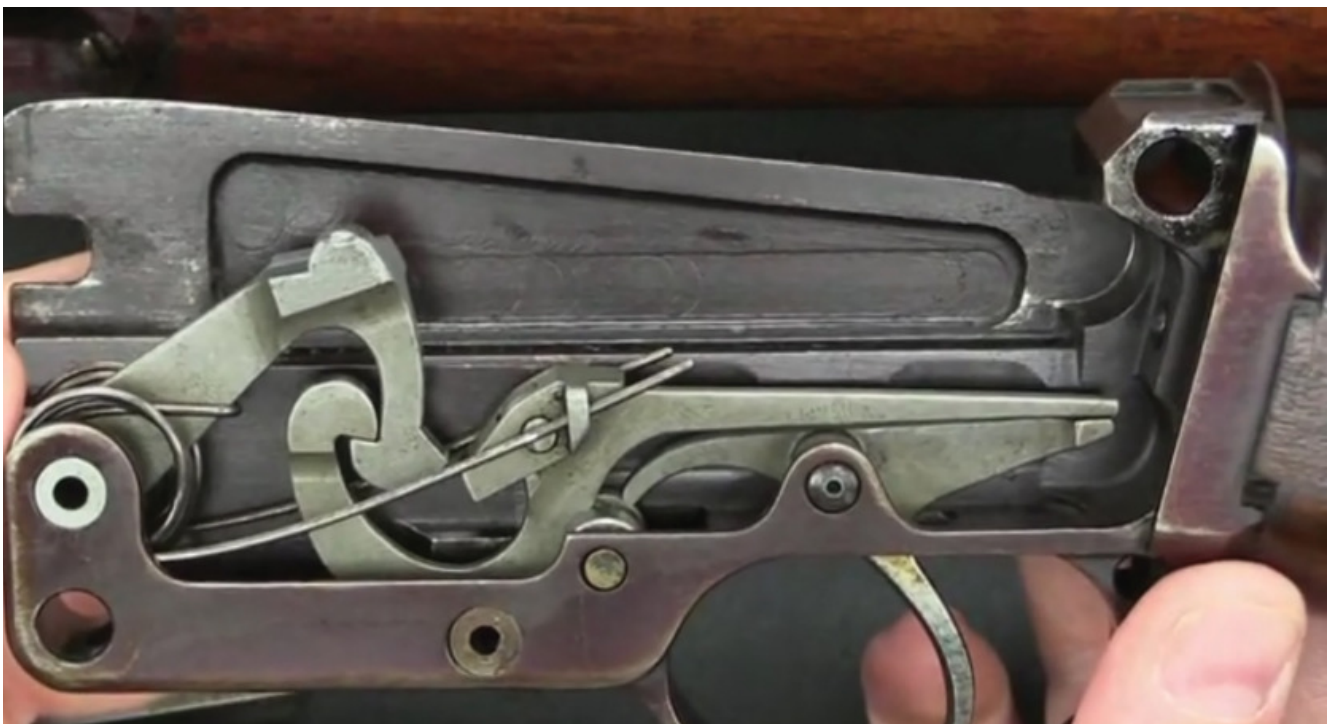
Pic. 13 Czechoslovak ZH-29 rifle (trigger system)
