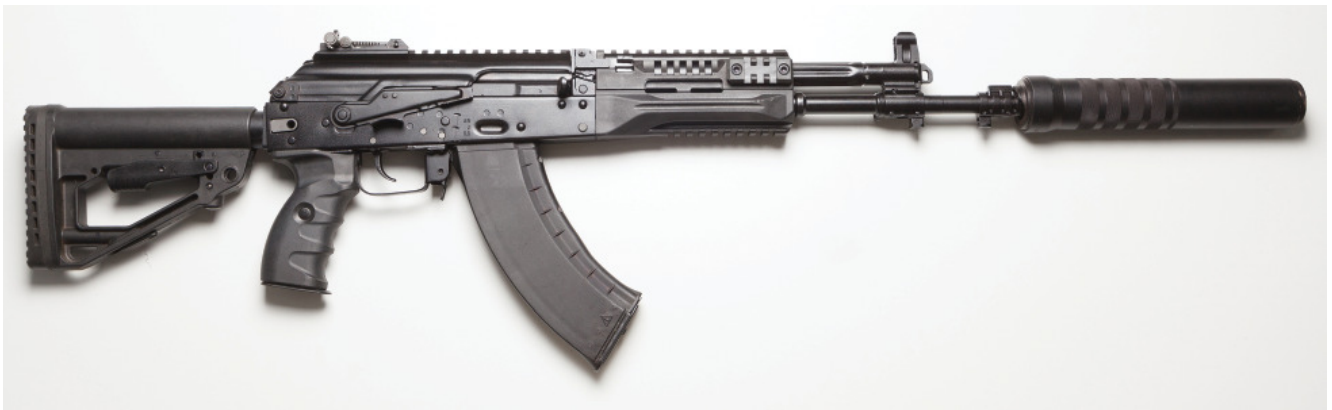
Pic. 31 7.62x39 mm version of the new AK-12 is known as AK-15. Shown here with tactical sound suppressor for Spetsnaz use.
