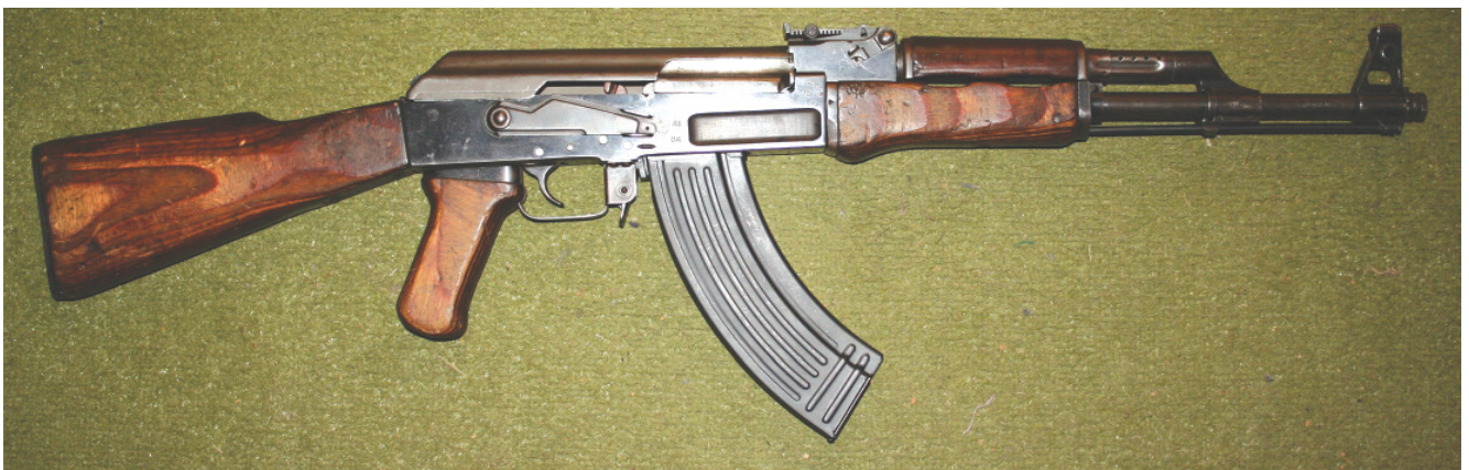
Pic. 12 Another early AK with machined receiver
